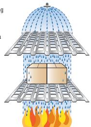
Punch Deck's open surface area allows sprinkler water through to lower levels.
